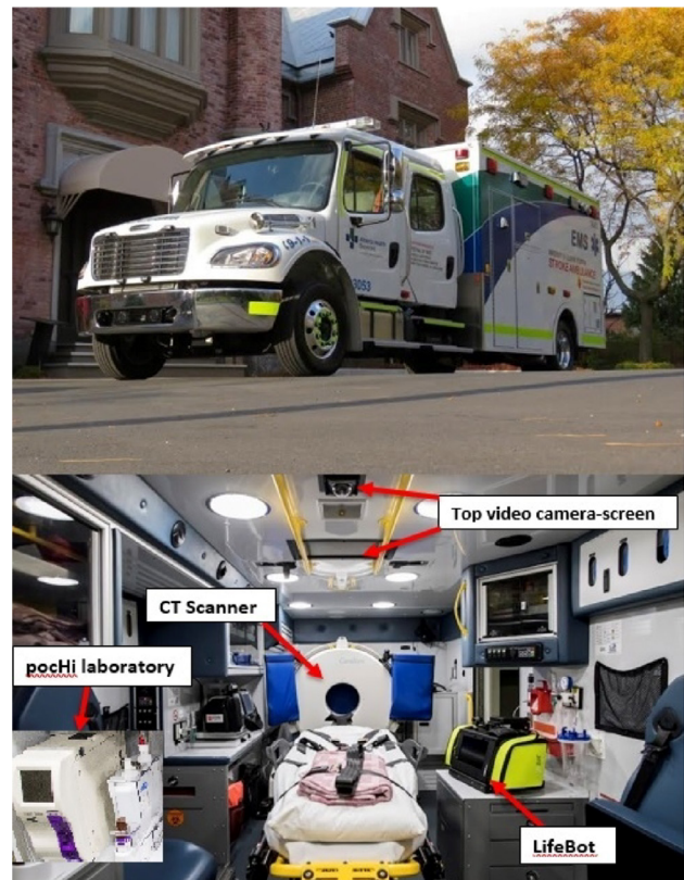
Figure 1 Mobile stroke unit based at the University of Alberta Hospital in Edmonton. The ambulance is equipped with a CT scanner, ‘point-of care’ laboratory and telemedicine equipment. The personnel deployed include one stroke fellow, two paramedics and a radiology technologist.
